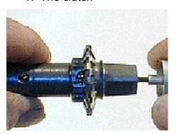
The heart of the **speed-drive** gearing system is the clutch, which is switched by pushing the gear shift button either on the left or on the right side.
