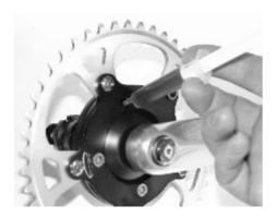
When assembling, we lube the **speed-drive** with a basic quantity of MoS2-grease, which is good for at least 2'000 - 3'000 miles.
