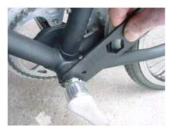
After several thousand miles, please check for bearing play. The chainring must not have any play along the spindle axis. If there is any play, slightly tighten the self-locking nut on the left end of the axle. Never tighten the nut too firmly. Some play between the cranks and chainring in the direction of crank rotation is normal and necessary for proper engagement of the gears after switching.
