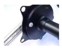
When assembling, we lube the *high-speed-drive* with a basic quantity of a special grease, which is good for at least 2'000 - 3'000 miles.
