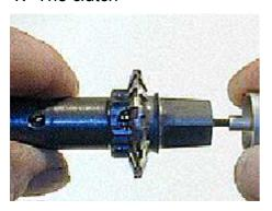
The heart of the *mountain-drive* gearing system is the clutch, which is switched by pushing the gear shift button either on the left or on the right side.
