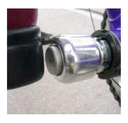
It's so easy: push with the heel of your shoe either on the right or on the left side of the axle on the push button to change from high to low gear or vice versa! That's all!
